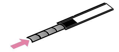
4 If you are scanning a strip of negatives with fewer than four frames, insert the negative light shield after the negative strip. See the icon on the negative holder for assistance.
